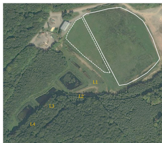
Fig. 1 The Etueffont landfill with lagooning ponds (L1: sampling pond, L2, L3 and L4) and location of old landfill (OL) and new cell leachates (NC) (top). Aerial view of the landfill (bottom)
